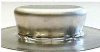
圖5：斜倒形狀試驗成品（來源：Embodied Computation: Exploring Roboforming for the Mass-Customization of Architectural Components）
