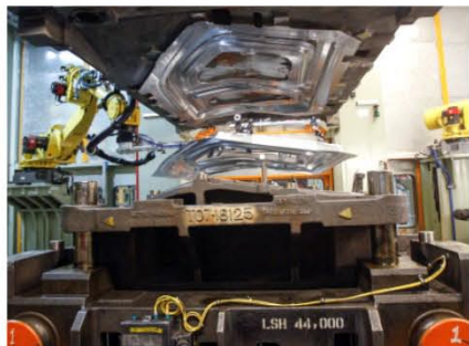
圖5：斜倒形狀試驗成品（來源：Embodied Computation: Exploring Roboforming for the Mass-Customization of Architectural Components）
