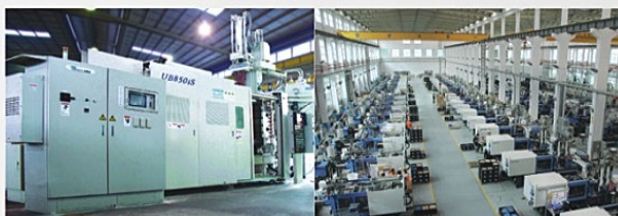
850 Cold Chamber Die Casting with Auto Extractor & Spraying | 850噸冷室全自動壓鑄機
