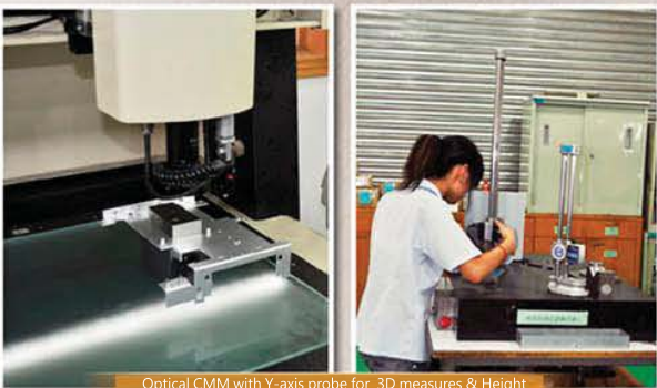
Optical CMM with Y-axis probe for 3D measures & Height Gauges 光學三次元檢測機械
